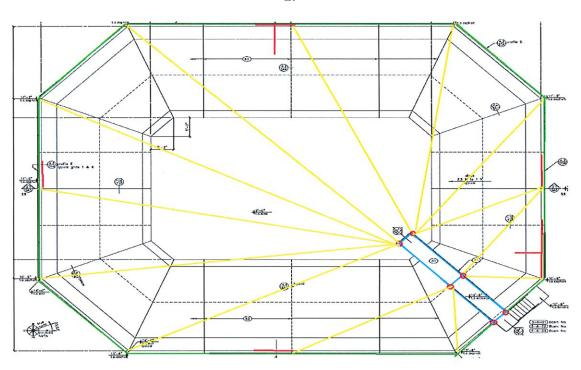
Red circles depict pole placements U-bolted to existing walkway guardrails. Blue lines depict cable framework to preserve service access to elevated walkway. Yellow lines show radiating support cable frameworks. Green lines show perimeter cable frameworks.
