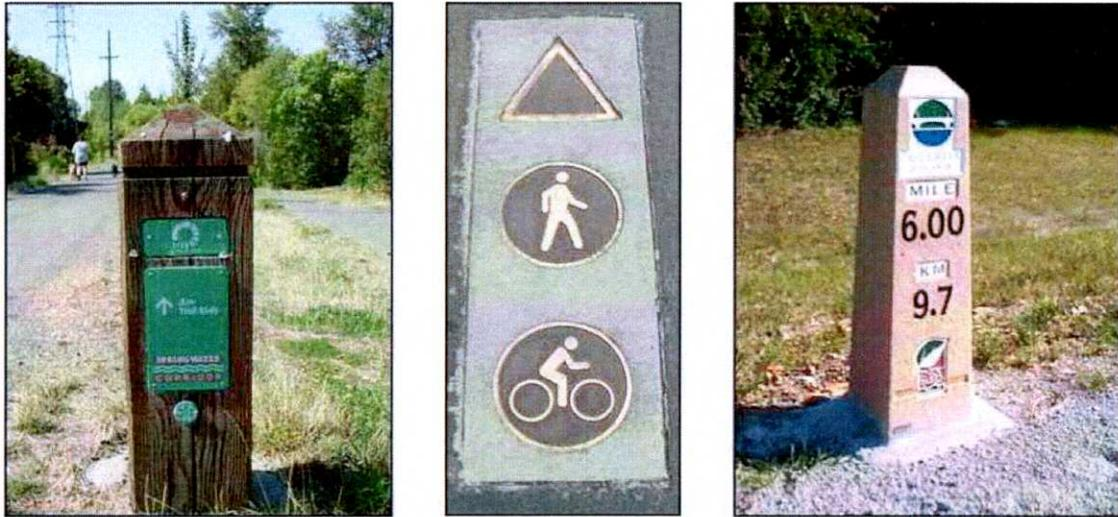
Figure 8. Bollards with Directional Information
