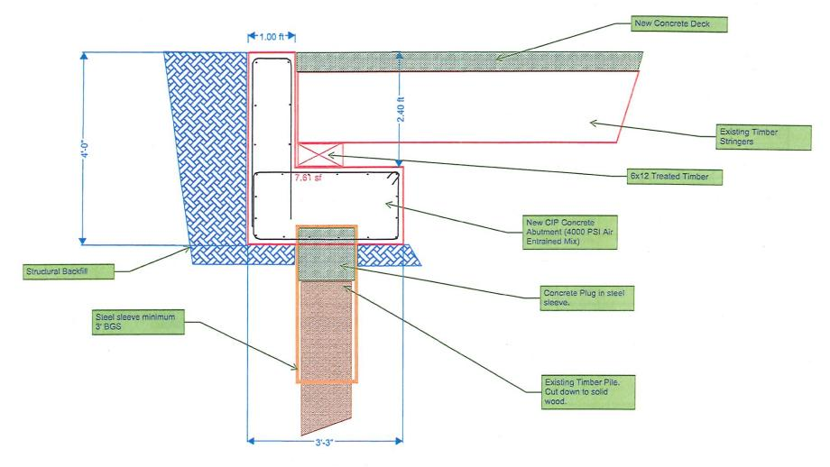
New Concrete Abutment Concept NTS
